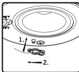
10. Attach grille safety clip by placing the large end of the clip over snap-fit post (1), gently press grille into place. then sliding clip until small end snaps into place around post (2).
